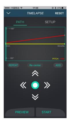
5 Tap 'SETUP' to set 'Shutter Interval', 'Shutter Duration' (shorter than 'Shutter Interval'), 'Target Clip FPS' and 'Target Clip Length'.
