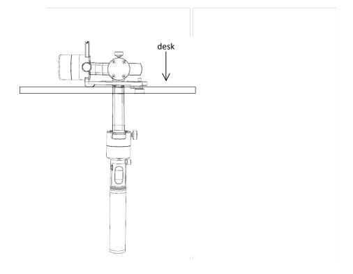
Here is a recommend position for accelerometer calibration.
